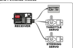
Install the Receiver in your model using double-sided Velcro. Velcro will hold the receiver in place and protect it from vibrations. Mount the antenna up and away from the vehicle in an antenna tube. The higher up the antenna is, the better signal it will receive.
