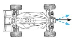
The steering trim is used to adjust the steering setting so that the car moves in a straight line without using the steering wheel to compensate.
