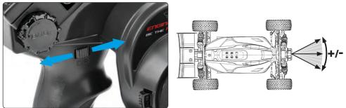
Use this function to adjust the steering travel of your model. If the model understeers while cornering, add steering by turning CW of the D/R button. When the model oversteers, take away steering by turning CCW of the D/R button.
